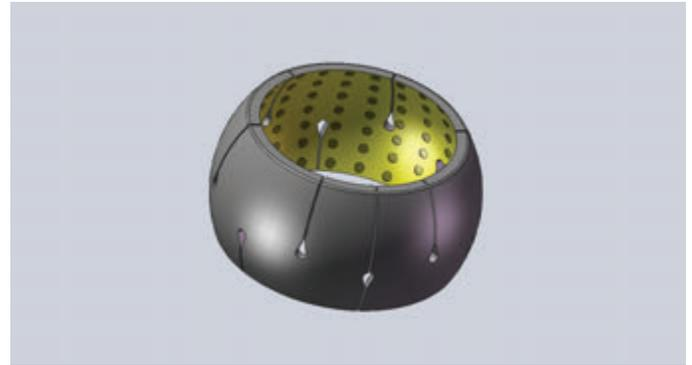
Additionally, due to notch and load effect present at the end of the spherical zone in the structure, bearing material is subject to deformation in time. Oscillation angle during operation of V stay arm is extended thanks to ‘teflon bearing’. Thus, load bearing capacity per unit surface is increased and oscillation angle is increased from 44° to 50° to offer a more flexible action for V stay arm.
